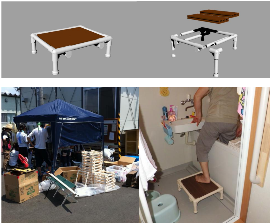
Figure 4. CG of Designed step ( upper Left), and its construction ( upper Right), on-site service ( lower left) and one trying step for Bathtub ( lower right)
