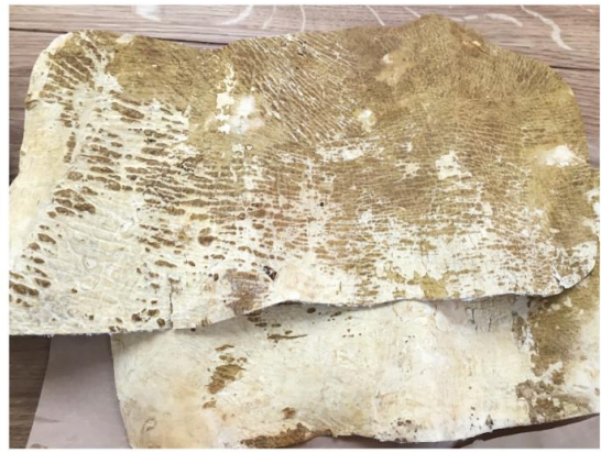
The mycelium is dried slowly to form a leather-like surface texture
