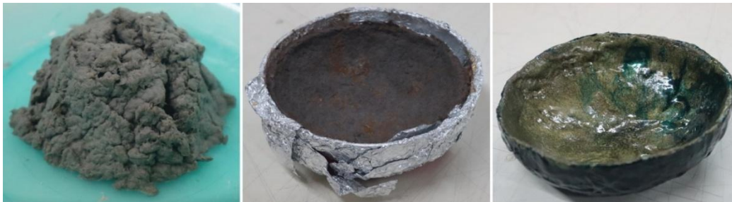
Figure 20: Paper pulp, Dried Paper Mache bowl, Final Paper Mache bowl coated with lac (left to right.)
