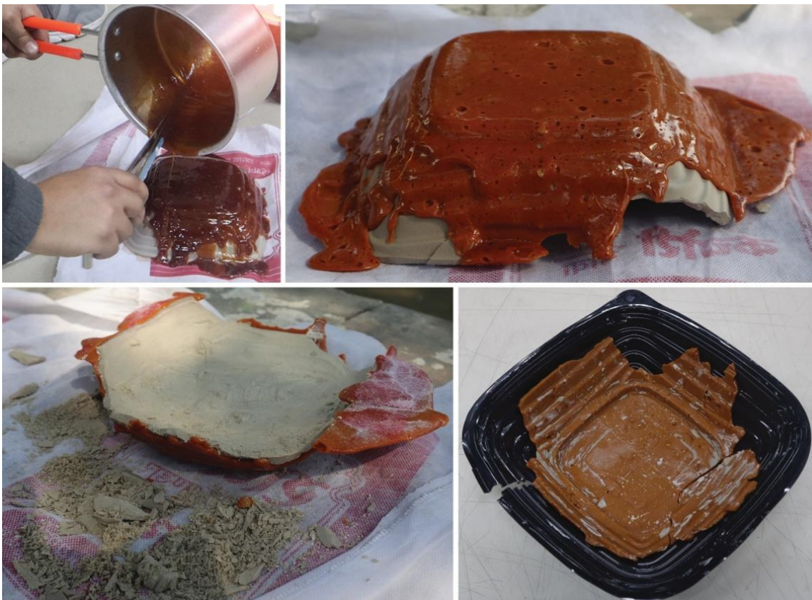
Figure 10: Casting with lac using POP mould.
