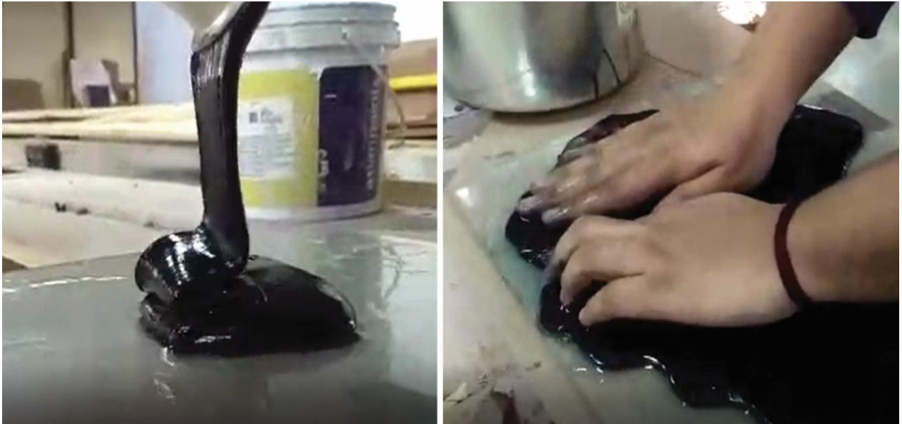
Figure 14: Pouring and spreading molten lac.
