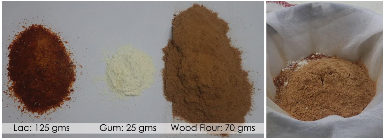
Figure 15: Preparing the mixture of lac, gum and wood flour.
