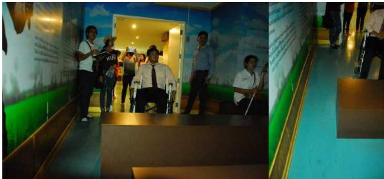
**Figure 9: Wheelchair testing can't access to exhibition area at 3D media room. Because of obstructive from furniture inside room, the way are narrow as well as non-point of rest for wheelchair.**
