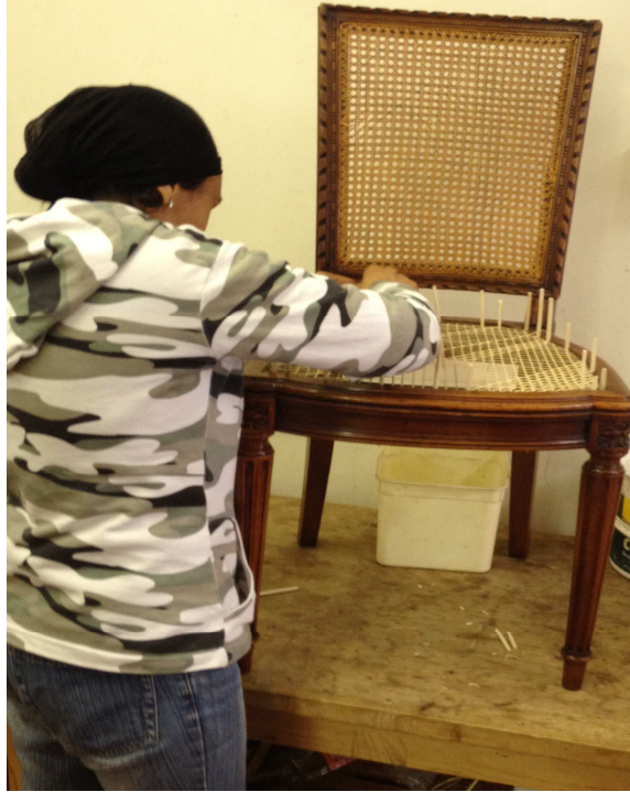
Figure 1: Crafter in the re-caning department repairing a chair. Source: Munyai (2013).
