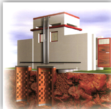
(c) View of toilet block with soak pit
