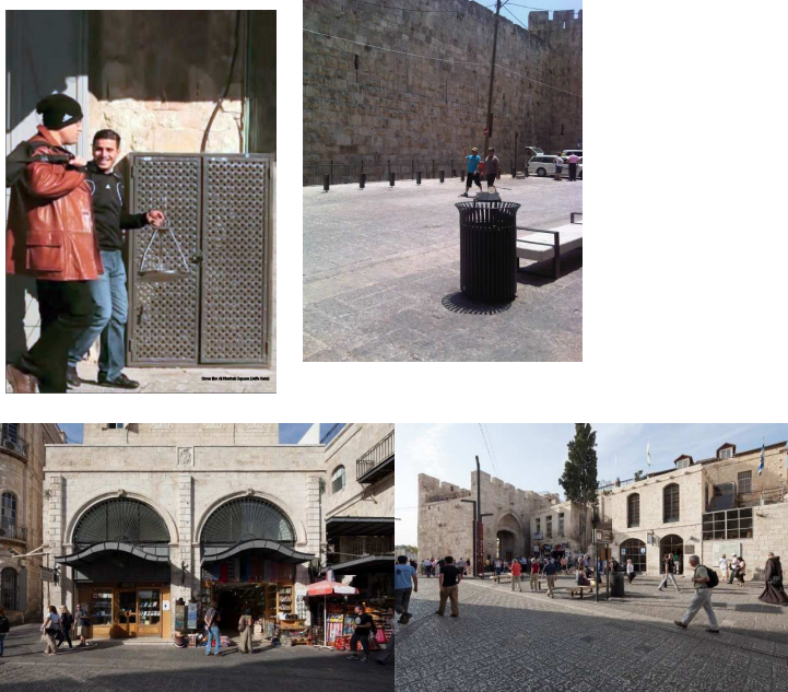
Figure 11: Modern fixtures such as the poles, garbage bins and benches were chosen to contrast with the old style oriental design of the buildings. The newly designed infrastructure cabinets within building facades resemble the ancient Mashrabiya 18 design style in nature and appearance but are based on a modern idea (IMSegev-"Segev Twist") of metal that looks woven even though it is only slightly curved.
