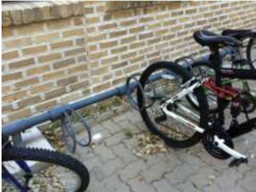
***Semi-toast: this type of racks is using two loops to hold the wheels. Even though racks that not provide support for bike frames are not recommended, (APBP, 2002) this is still one of the most commonly found bike racks on campus. They are representatives of old-fashioned bike racks.***
