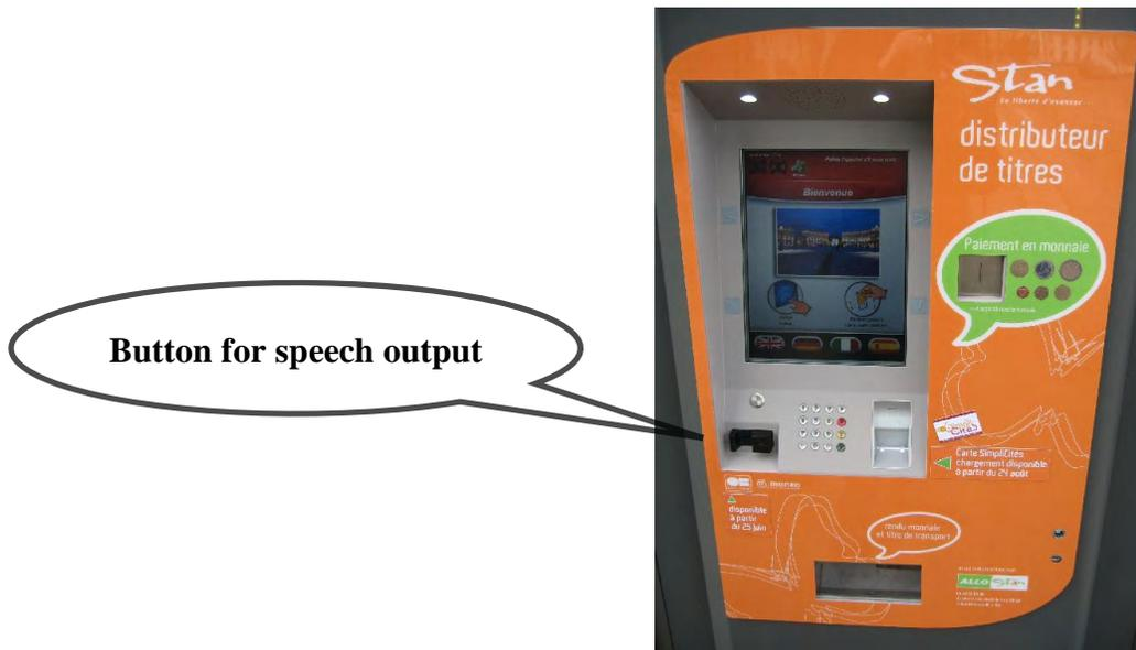
**Figure 9: example of accessible ticket vending machine implemented in France (source Certu, 2011)**
