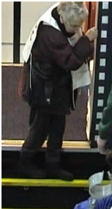
**Figure 4: contrasted step noses and handholds on a coach door simulation (Atkins, 2004)**
