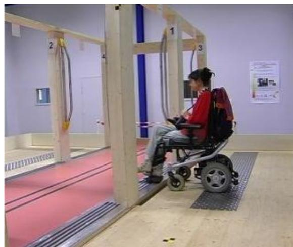
***Figure 2: Laboratory tests – level access for wheelchair users (Grange-Faivre, 2013)***
