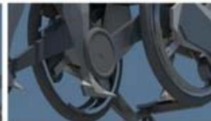
SUSPENSION CONNECTED REAR WHEELS EASE THE TASK OF UP-HILL CLIMB
