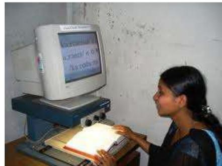
**o Large magnification devices such as closed-circuit television magnifiers (CCTV). This system employs a video camera lens to enlarge text from three to thirty times normal text size**
