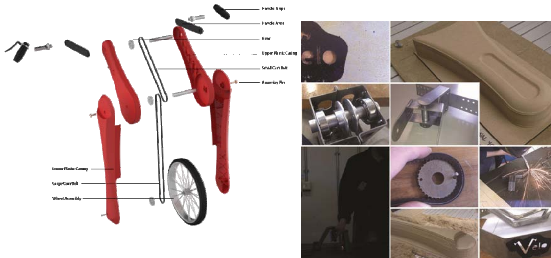
Figure 19: Shows a conventional DFMA approach to a principle-proving prototype. (Designer: Mark Wafforne)
