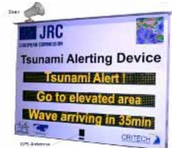
***The JRC Tsunami Alerting Device (TAD) is activated by new software that quickly calculates the estimated wave height and travel time.© EU, 2011***
