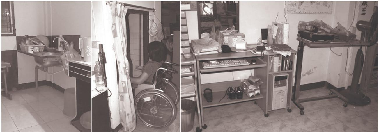
**Figure 2 Home furniture modified to fit in with Tum's requirements: (from left to right) the wash basin lower supports have been removed; at the entrance to the bathroom a plastic curtain has replaced the usual swing-door; and desks that are mobile and cabinets with wheels are used instead of fixed furniture.**
