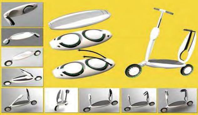
The idea was to design a compact, easy to handle, economic, light weighed and eco friendly portable mobility device which can be carried like a bag pack and used like an electric scooter.
