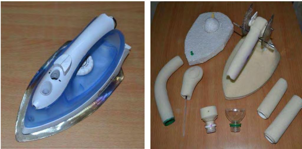
**An experimental setup was made up to study the grip parameters. The set up comprised of an iron with an adjustable hinged handle in vertical plane to study effect of handle inclination, an iron with a handle connected to main body with a spherical joint to study azimuthal plane deviations and threaded joints for handles to allow axial rotations and for changing of handles with different curvatures.**
