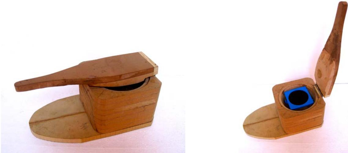
*Longer lever arm with support at the base and integrated bowl; allowed any number of trials while using without the pressure of chopping in one go*
