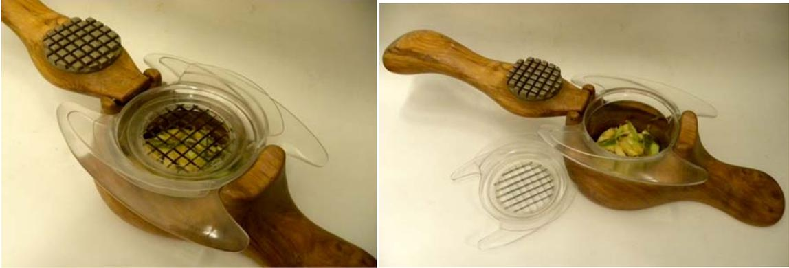
*The bowl and blade plate in place when the vegetable/fruit is kept in the depression on the blade plate and force is applied from top; the blade plate out of the bowl once the chopping is done*
