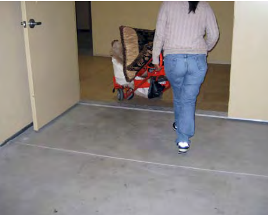
As Dana points out, the wide entrance with level floor makes it easy the building for everyone.
