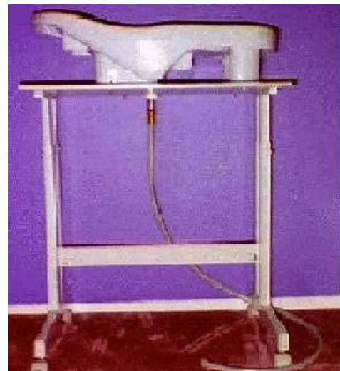
Figure2. Commercial tub attached to computer table. Drain is connected to dishwasher hose.
