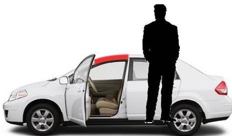
As indicated in the illustration, the roof restricts the natural movement during ingress and egress. One has to bend to accommodate the upper body. This exercise requires a certain amount of flexibility and strength of the body.
