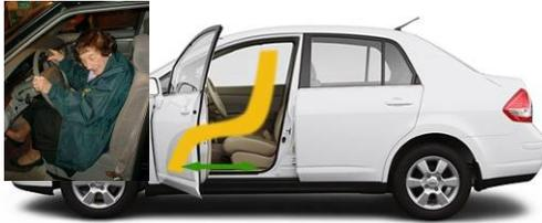
The position of the seat coupled with the position of steering wheel and roof provide a slanted opening for entry. This requires the body to slide in with the legs forward and the whole body's weight to be supported by the hands. It is a difficult exercise if the hand muscle is not strong enough.
