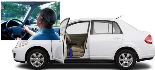
The seat height in cars and sedans are very low. This further aggravates the situation during ingress and egress. To sit down to such low positions and again rise up from it require strong leg and hand muscles. It also reduces the field of vision as the level of the eye is lower.
