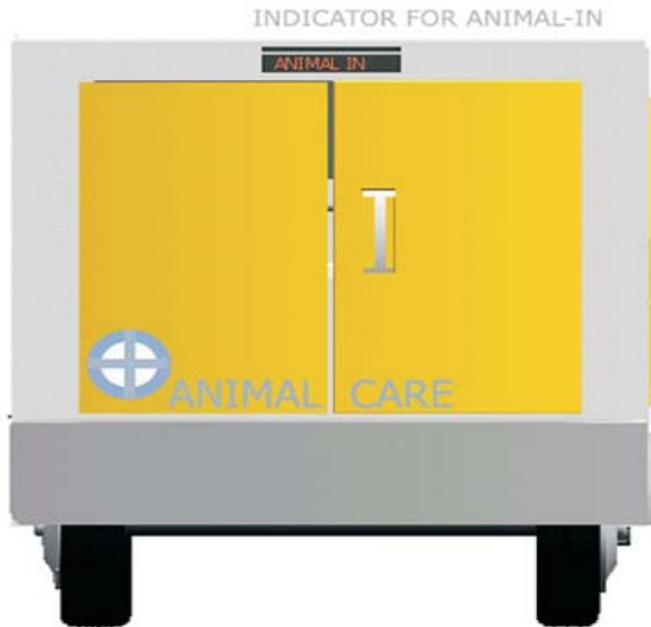
The pickup box has been redesigned for animal comfort, safety, and security. Additions include side ramps for loading & unloading the animal, special customized cages, storage provisions for water & medicines, ventilation, & foldable table for medical examination. Animal behaviour
