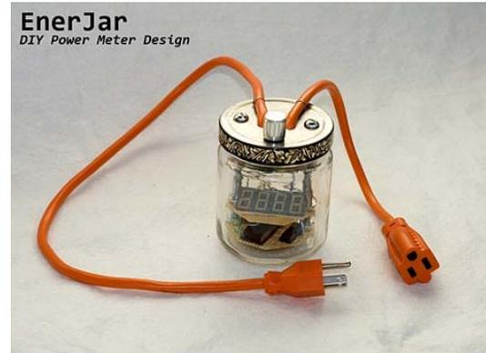
The EnerJar is an easy-to-build device that accurately measures the power draw of electrical appliances. The EnerJar was the winner of the Greener Gadgets design competition. The design is still being optimized, but preliminary schematics and source code can be found on this site by following the "Hardware" and "Software" links to the left.
