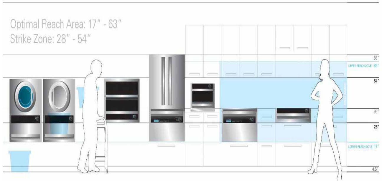
Fig. 5 Illustration of the optimal "strike zone" for access by all users
