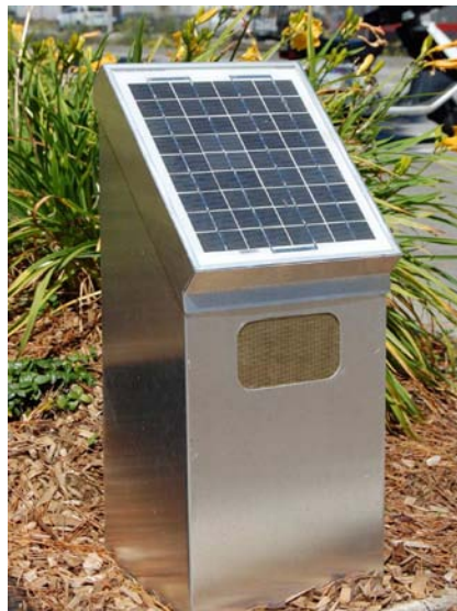
Figure 1 – An audible landmark on the university campus provides an additional source of wayfinding cues
