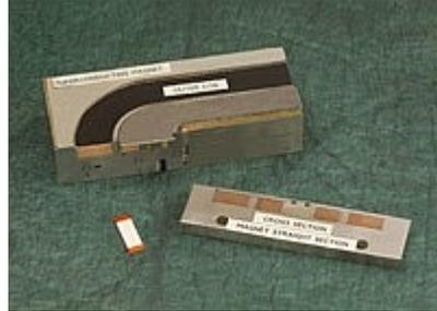
**The magnets consist of metal or ceramic superconductor coil windings made of very fine filaments. The required electrical insulation between the filaments is provided by glass filaments. In the case at hand, the superconductor is a ceramic and the glass filaments must be very thin.**
