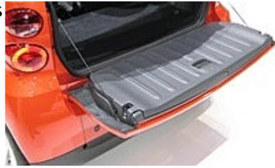
Compared to the previous solution, the parts meet higher rigidity and crash-resistance requirements, at 10% lower cost. Functional integration provides higher strength and additional storage area. The concept, which allows for great design freedom, uses low-cost materials (PP/glass fibre), but offers high crash resistance and lower weight compared to a metal solution.
