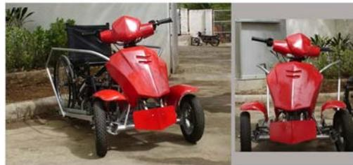
The Final prototype has been tested with the help of a user and the important finding was, that it need a little customisation in a vehicle so that it caters a particular kind of disability, and some training will be necessary before moving out on the roads.
