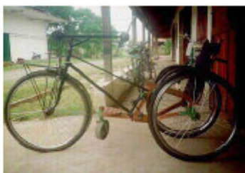
A wheelchair converted into a tricycle.
