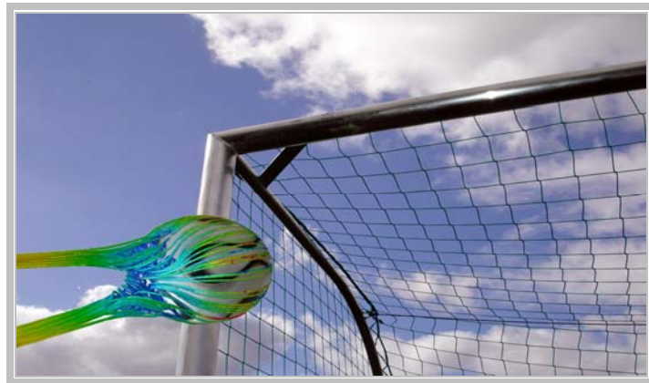
Figure 1: Velocity pathlines around the new World Cup ball
