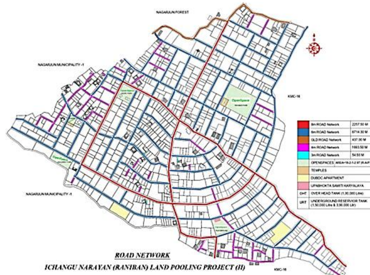
Fig. 6.1 The layout plan for Ichangu Narayan land pooling project
