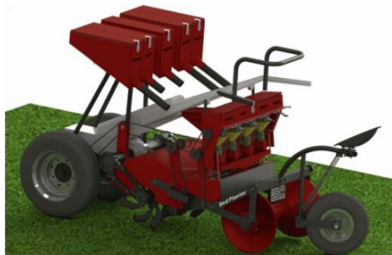
Fig. 2 CAD model of the bed planter attachment
