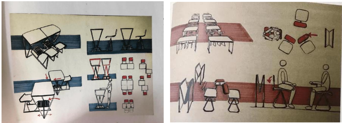
Figure 15: Chairs are fixed to the table through a track. Which help the chair slide in the table. Bag storage is underneath the table. Different configurations are possible.
