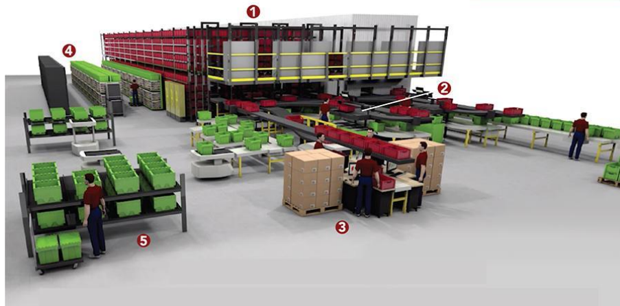
Fig.16 - MFCs combine robots with human labor to speed up delivery at a reduced cost. Source: MMH (CB Insights, 2020)
