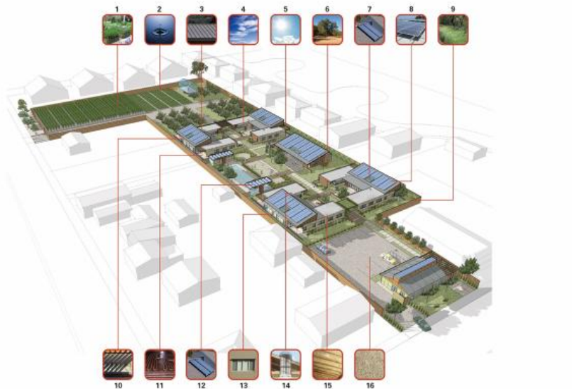
SUSTAINABILITY DIAGRAM 1 ORGANIC FARM 2 IRRIGATION WELL 3 COOL ROOF 4 NATURAL VENTILATION 5 DAYLIGHTING 6 DROUGHT TOLERANT PLANTS 7 SOLAR HOT WATER PANELS 8 SOLAR PV PANELS 9 STORMWATER FILTRATION BIO-SWALE 10 SUN CONTROL 11 RADIANT FLOOR SYSTEM 12 POOL SOLAR PANELS 13 HIGH PERFORMANCE WINDOWS 14 SOLAR TUBE SKYLIGHTS 15 HIGH R-VALUE EXTERIOR WALLS & ROOF 16 PERMEABLE PAVING
