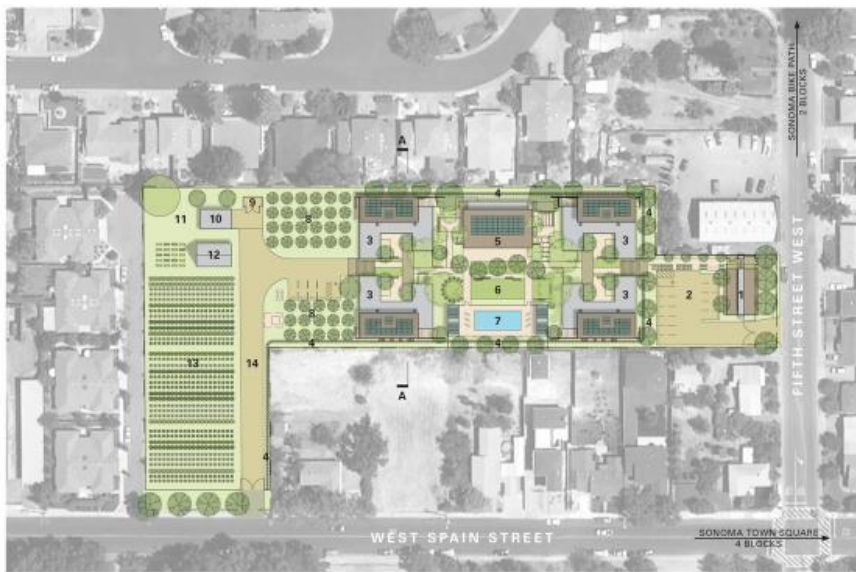
SITE PLAN 1 WELCOME BUILDING 2 PARKING 3 HOUSE 4 STORMWATER TREATMENT BIO-SWALE 5 COMMUNITY CENTER 6 THE COMMONS: PLAZA & LAWN 7 THERAPY POOL & SPAS 8 ORCHARD 9 TRASH 10 STORAGE BUILDING 11 IRRIGATION WELL 12 GREENHOUSE 13 ORGANIC FARM 14 FIRE ACCESS ROAD
