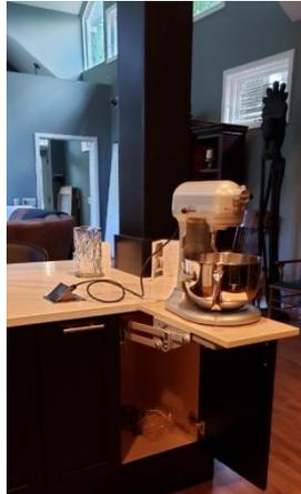
**View of KitchenAid mixer in the raised position. A KitchenAid mixer is embedded in a base cabinet that stores and raises this heavy mixer to a height that a seated baker can work with it and also easily store it below when finished. The mechanism that raises it handles all of its very heavy weight. The electrical socket to the left is embedded into the counter top and is a pop-up type.**
