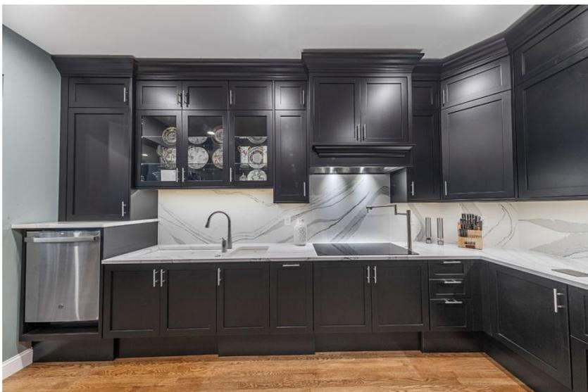
**View of main kitchen sink. Items underneath this sink are neatly stored in baskets so that if this space needs to be opened up for a seated cook they are easily removed. Raised dishwasher is to the left. A raised dishwasher is easily used by a seated cook, but incredibly convenient for a standing cook! It was designed to be**
