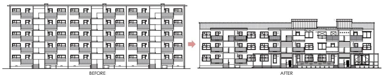
Figure 9: Building No.28 south façade level subtraction
