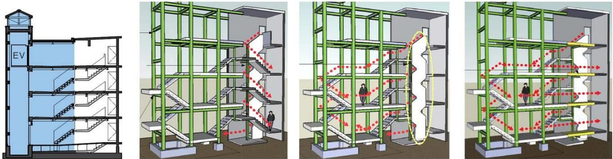
**Figure 7: Elevator addition system. Installation works can be done without interrupting residents' activities (Source: UR)**
