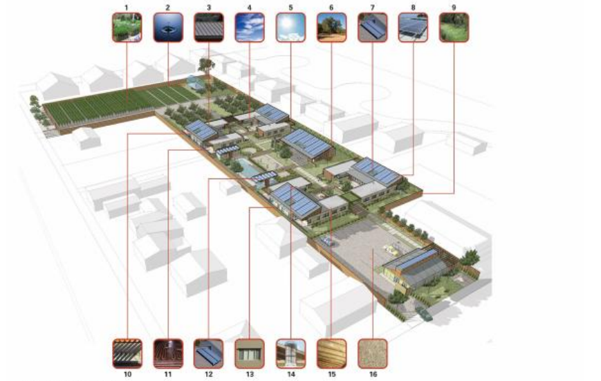
SUSTAINABILITY DIAGRAM 1 ORGANIC FARM 2 IRRIGATION WELL 3 COOL ROOF 4 NATURAL VENTILATION 5 DAYLIGHTING 6 DROUGHT TOLERANT PLANTS 7 SOLAR HOT WATER PANELS 8 SOLAR PV PANELS 9 STORMWATER FILTRATION BIO-SWALE 10 SUN CONTROL 11 RADIANT FLOOR SYSTEM 12 POOL SOLAR PANELS 13 HIGH PERFORMANCE WINDOWS 14 SOLAR TUBE SKYLIGHTS 15 HIGH R-VALUE EXTERIOR WALLS & ROOF 16 PERMEABLE PAVING
