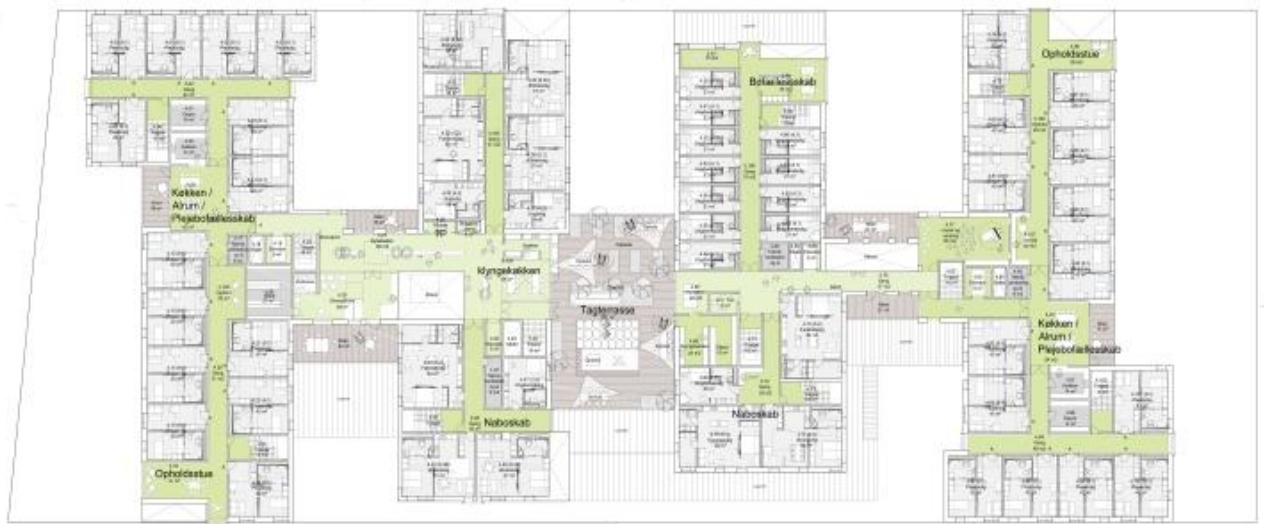
Picture 6- A typical floor plan depicts the relationship between dwelling units (white) to their semi-private circulation spaces within each "house" (dark green), which links to the semi-public common spaces adjacent to each "house" (light green). Outdoor public spaces are indicated in brown.
