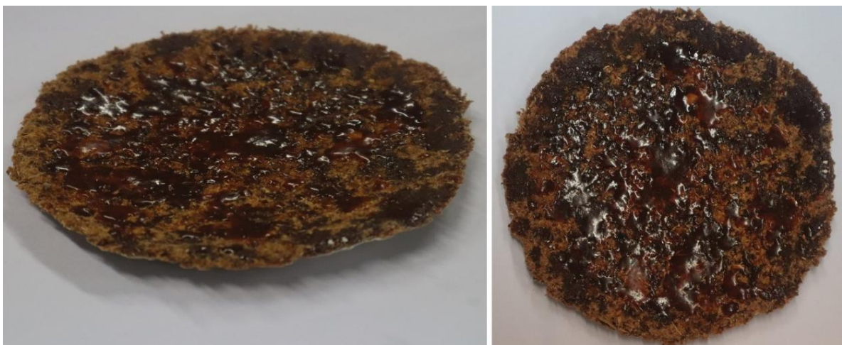
Figure 17: Sheet of lac and wood mixture.
