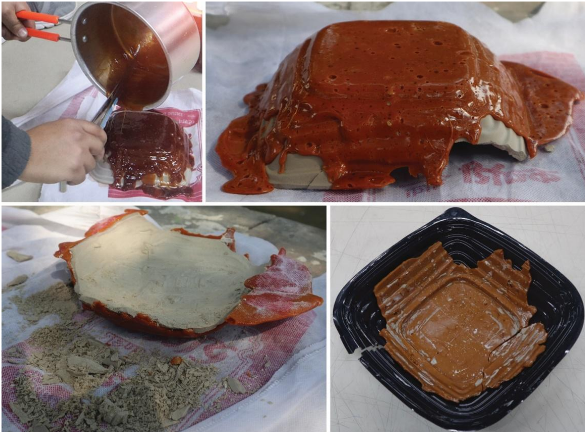
Figure 10: Casting with lac using POP mould.
