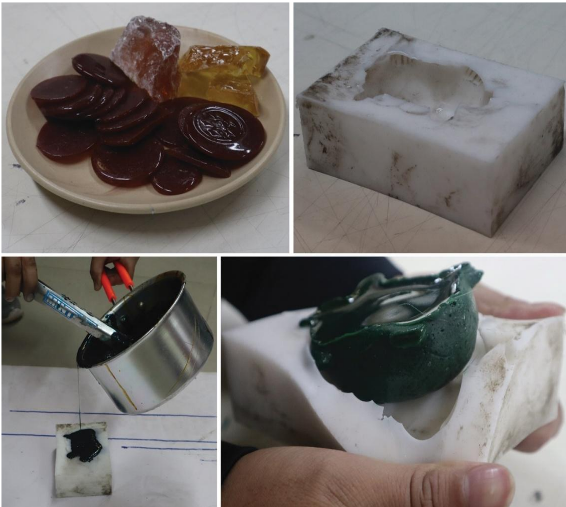
Figure 12: Mixing equal amount of lac and Berja gum by weight (top left), preparing silicon mould for casting (top right), Pouring molten lac in silicon mould (bottom left), taking out the artefact out of mould (bottom right)
