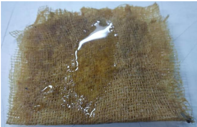
Figure 19: Cotton cloth soaked in liquid lac solution displaying properties like waterproofing.
