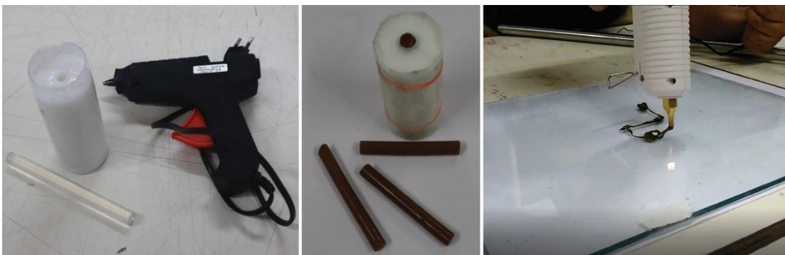
Figure 21: Silicon mould used to make lac stick, using lac stick with glue gun (Left to right).
