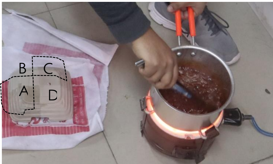
Figure 9: POP mould on left being prepared for casting.
