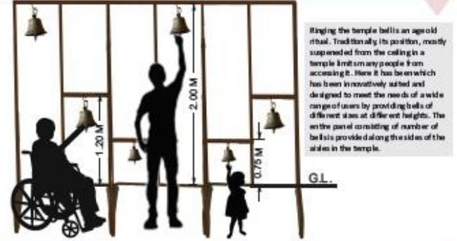
Ring the temple bells is an age old ritual. Traditionally its position, mostly suspended from the ceiling in a temple limits many people from accessing it. Here it has been which has been innovatively suited and designed to meet the needs of a wide range of users by providing bells of different sizes at different heights. In the panel consisting of number of bells provide along the sides of the area in the temple.
