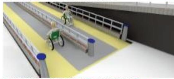
VIEW SHOWING GUIDED TRODS ON THE RAMP, TACTILE BOLLARDS AND RAILINGS
