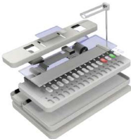
Caption: Exploded View of the EVM-VVPAT Hybrid
