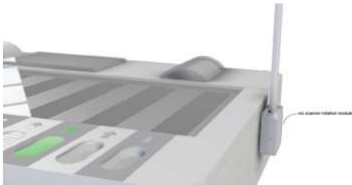
Caption: Iris Scan Module of the EVM-VVPAT Hybrid
