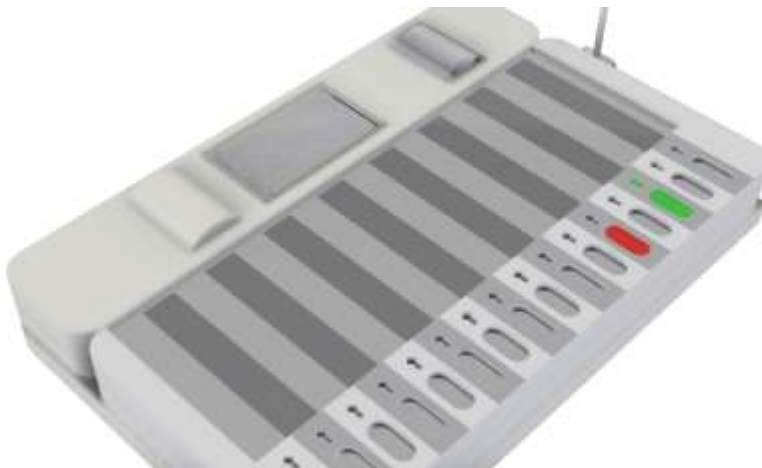
Caption: Visual Cues on the Interface of the EVM's Candidate-Party Panel (to lessen the voter's cognitive load)
