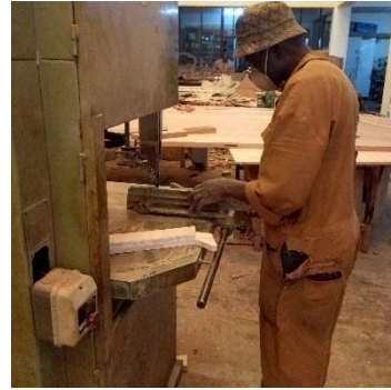
Fig 24: Carpenter using band saw for small pieces Source: the researcher
