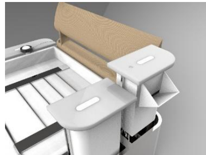
Figure 4 left hand side chambers (water inlet)
