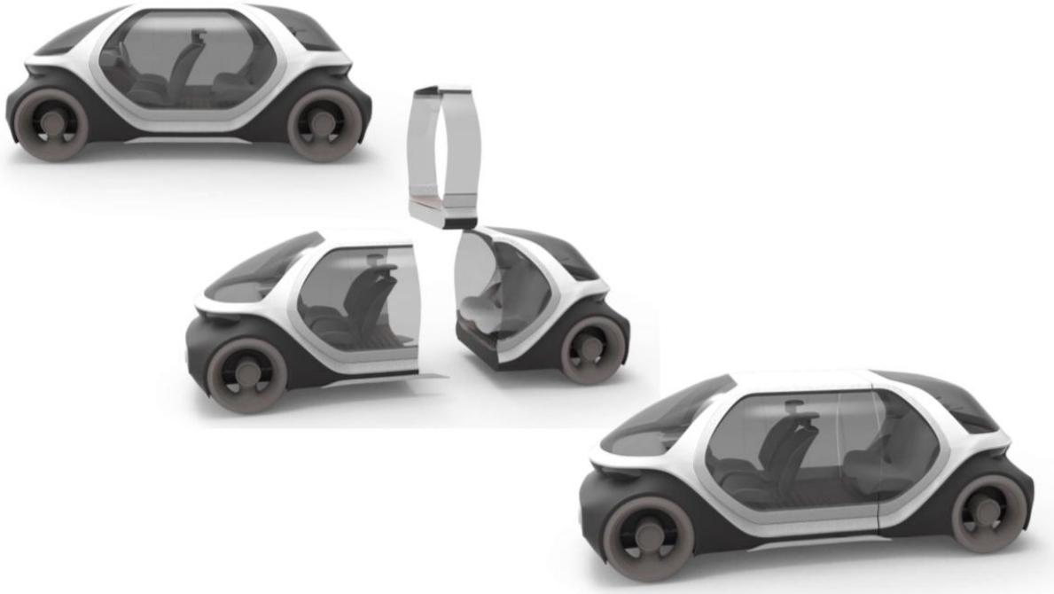
**Figure 11: frame and exterior modules to allow extension in length (source: author)**
