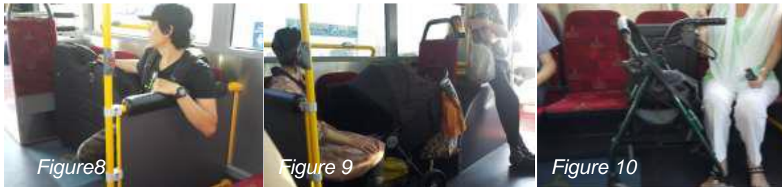
Figure 8-9-10 Bus with inclusive interior design, other good example of universal access # equitable # wheelchair and baby-stroller lots are carefully provided prior for disadvantaged, with flexible in use, if no, adaptable for general people.
