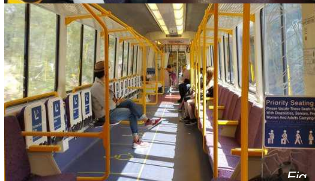
Figure 6-7 Train with inclusive interior design, other good example of universal access # equitable # wheelchair and baby-stroller lots are carefully provided prior for disadvantaged with flexible infrastructure, adaptable for general people. Brisbane, Gold Coast train.
