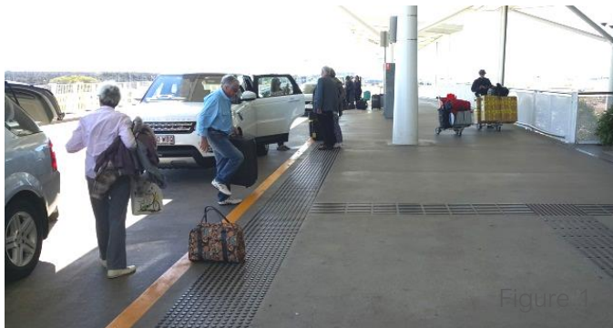
Figure 1 Illustrated drop off area of the airport with various inclusive devices installed such as hi-intensity strip, Braille pavements and ramp slope.
