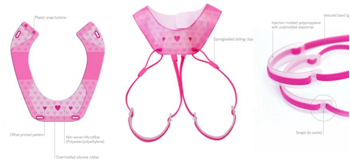
Fig 21. Final Product "H": Manufacturing details
