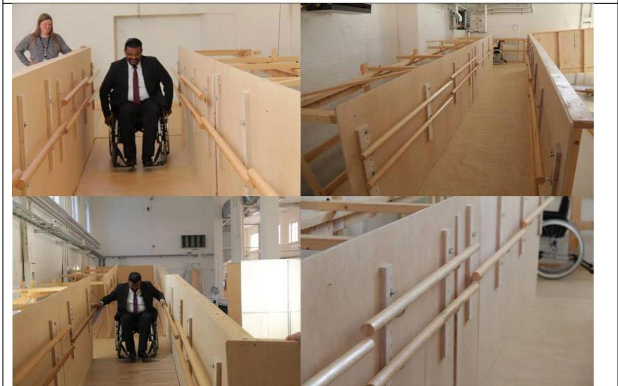
***The study of ramps with different gradients, varying surfaces with different materials and varying heights of handrails.***
