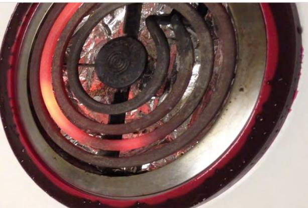
**Image 7:** Prototype made of silicone rubber is changing color from dark brown to red.
