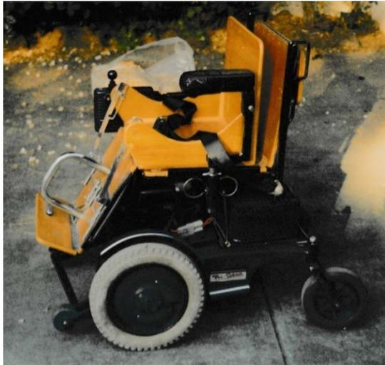
The seat is 33 cm high and supports my back. The seat and leg support area is jointed at equivalent points to my knees and ankles. The first and second jointed pieces are each 38 cm wide and 33cm long. When the leg support is extended the whole length is 75.5 cm long.
