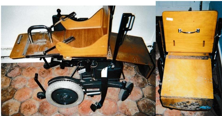
Behind the seat there is a handle which an assistant uses to pull me and the seat up the base board into a car. Underneath the wood seat are Teflon runners to assist the sliding process over
