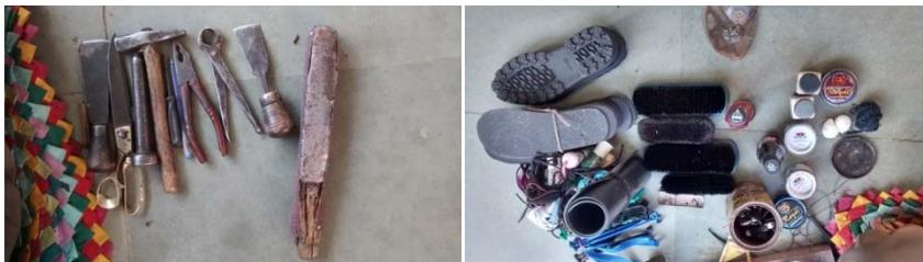
*Tools / Materials - Scissor, Hammer, Plier, Chisels, Emery paper on wooden bat, Screwdriver, Iron stand, Needle, Rubber soles, brushes, Adhesive, Laces, oil, nails, nylon thread*
