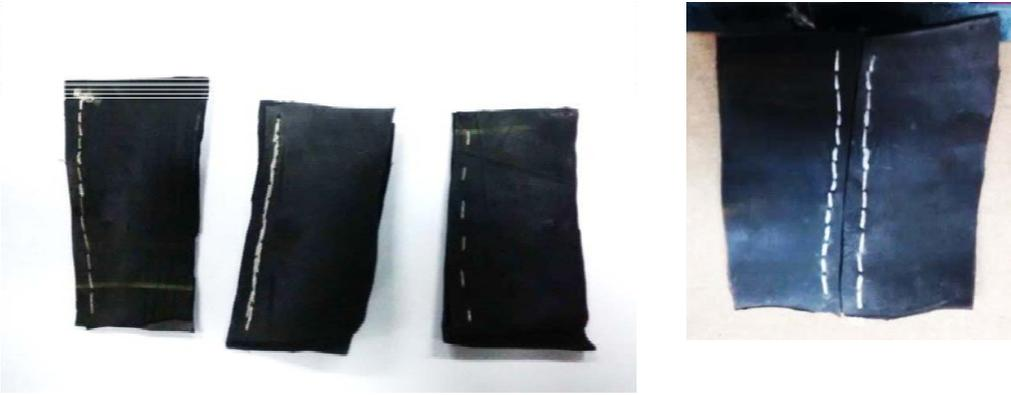
*Running stitch, double running, loop stitch and edge to edge stitching in swatches*
