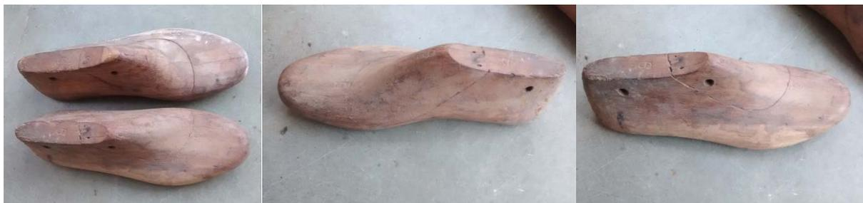
*Wooden shoe last used to make the shoe pattern for correct fitting*
